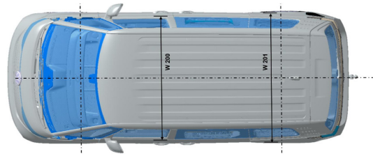
Fig. 1: Example vehicle dimensions of the ID Buzz People (acc. to DIN 70020, P2) The dimensions are given in the basic data table below.
